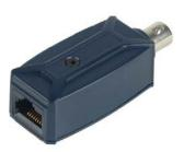
IP01 is a low cost and easy, speedy solution to allow you use existing coax cable to send IP camera signal. Used in pairs with your RG59 cable to exceed the IEEE 802.3 10BaseT NEXT specification. The working range could up to 200 meters at 10Mbps speed.
