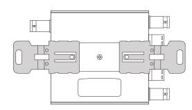
4. Fix the unit in the desired location with two screws.
